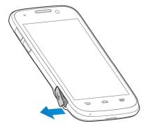
Connect the adapter to the charger/micro-USB jack. Ensure that the adapter is inserted with the correct orientation. Do not force the connector into the charger jack.
